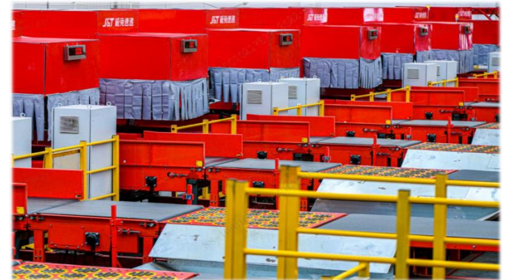
DWS and pivot wheel sorter: suitable for all sorting centers
