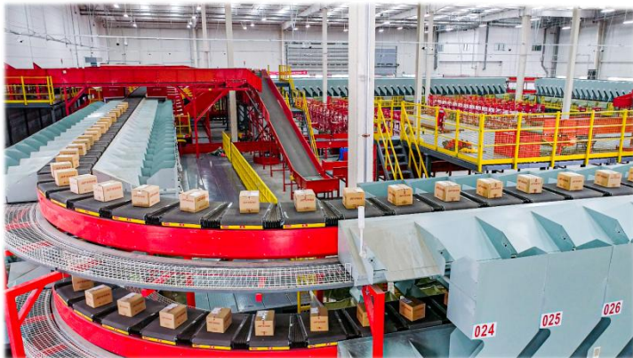
Cross-belt sorting line: suitable for sorting centers with large volume of small parcels
